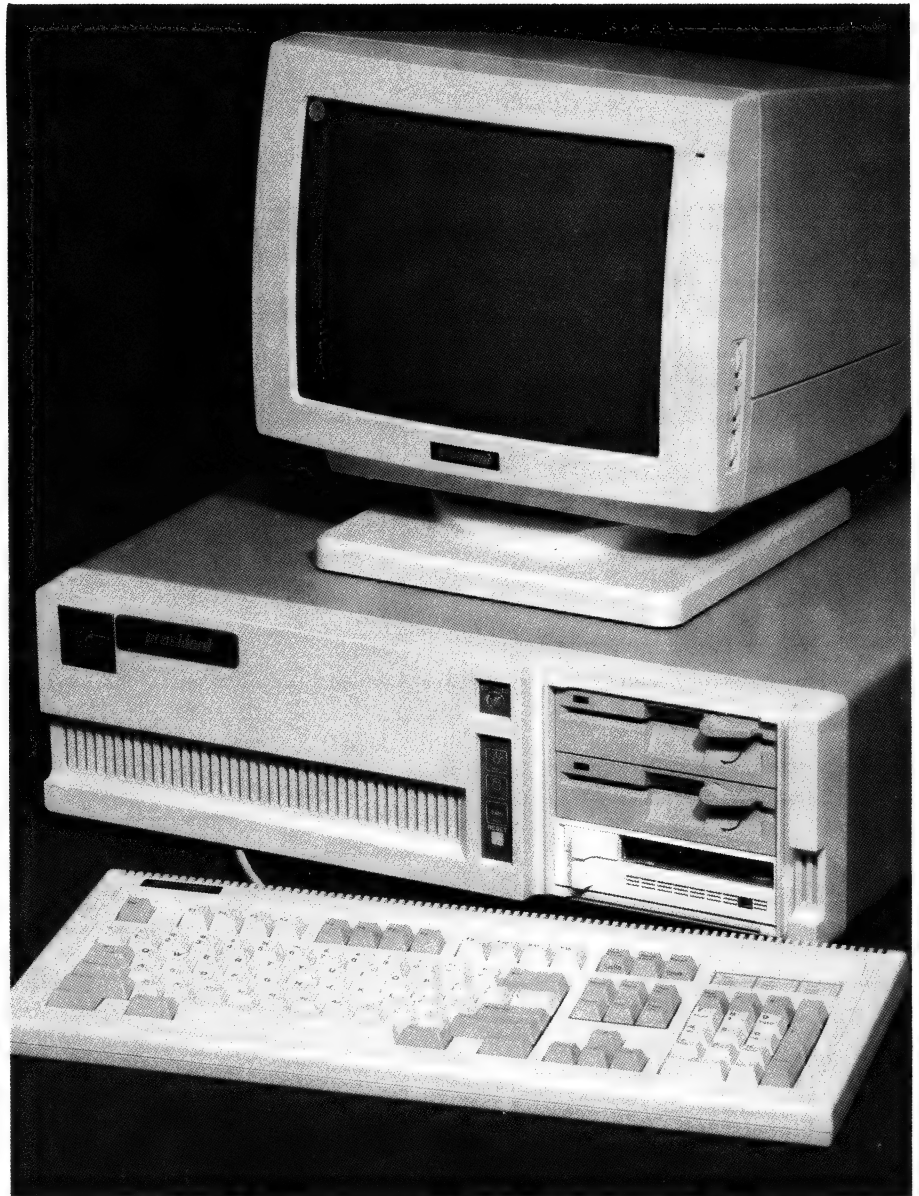
The President 286, shown here sporting two floppy drives, and a tape backup unit.
