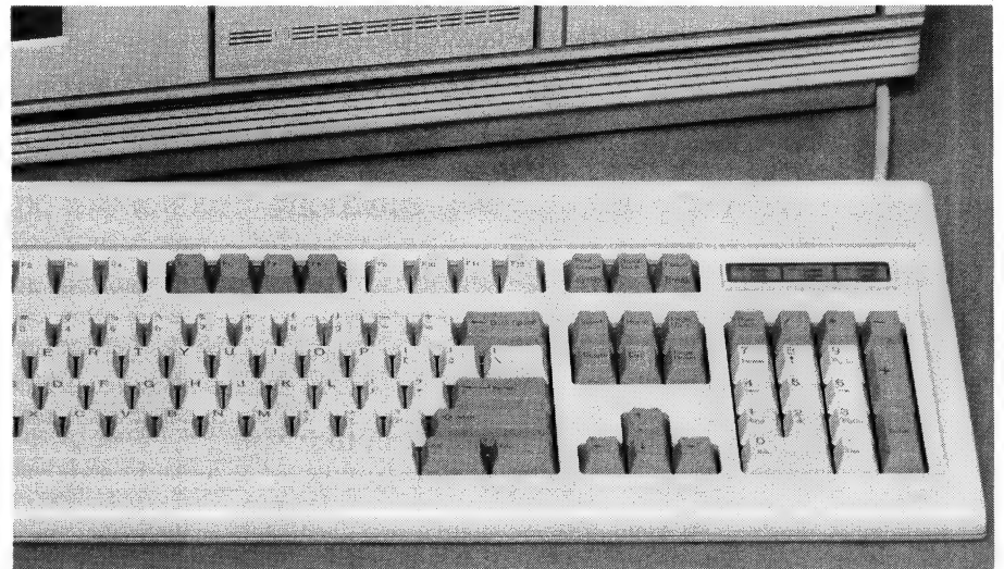
The Power Mate keyboard is ultra thin with 101 keys and a separate numeric keypad and a cursor diamond, as well as 12 programmable function keys.
